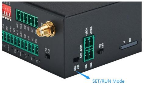
Connect the device to an external power and power on, switch the power switch to ON.
